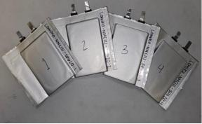
Lomiko graphite Half-cell batteries produced and tested by Polaris (SPG16 top, SPG20 bottom row) SPG20 sample from La Loutre has superior charging capacity compared to commercial graphite in the market today in North America.
