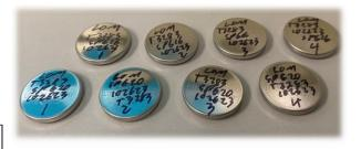
Lomiko graphite Half-cell batteries produced and tested by Polaris (SPG16 top, SPG20 bottom row) SPG20 sample from La Loutre has superior charging capacity compared to commercial graphite in the market today in North America.
