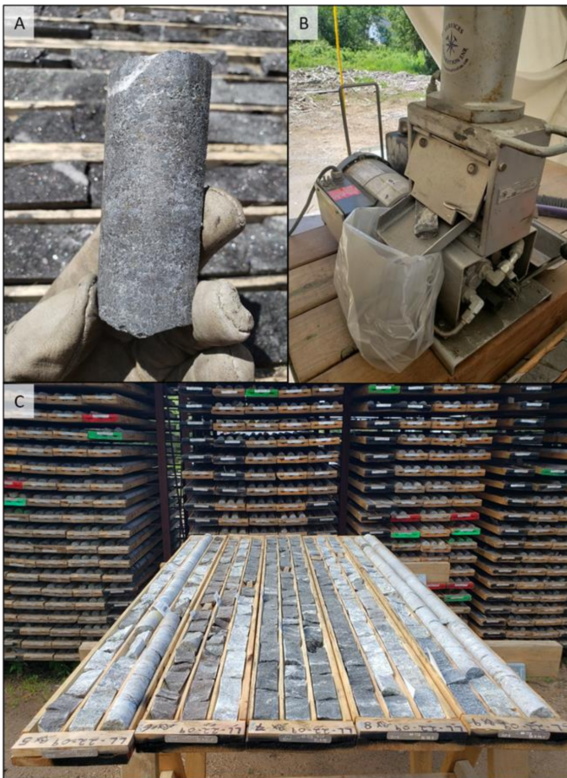
A) Mineralized drill core with millimetric graphite flakes from hole LL-22-032; B) Hydraulic core splitter; C) Photograph showing proper storage and labelling of the drill core boxes and sample tags still stapled in the boxes.
